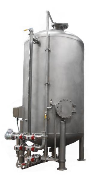
"Except on rare occasions, a Resin Softener should not be sized to regenerate more than once per day. A worst-case condition for feedwater quality should be used when sizing the softener capacity. It is common practice to oversize a softener by at least 10% to ensure that the bed will not be exhausted prior to regeneration."
