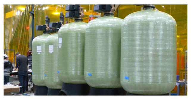
and magnesium ions with sodium, thus no calcium carbonate (CaCO3), Calcium sulfate (CaSO4) or magnesium hydroxide (Mg(OH)2) scale will form to foul the heat transfer surface areas, maintaining heat transfer efficiency and reducing downtime for cleanings. Resin softeners do not remove silica, however if the calcium and magnesium has been removed, silica scales will not form.
