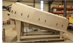
With its longstanding industrial experience, Nijhuis Industries has developed a cost-effective screw press system (NSP) to dewater sludge without high fibers or abrasive solids, including, both physical-chemical biological types of sludge.
