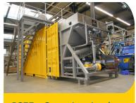
**ICFF** - Containerized DAF system based on a plug and play principle
